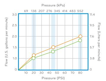
Oxygenics 1.8 GPM Oxygenics 2.0 GPM
