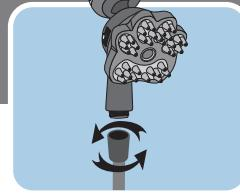
Sink adapter fits two common sizes of faucets after removing aerator:
